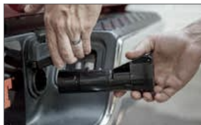
Insert Echo™ between the vehicle-trailer 7-way RV blade connectors
