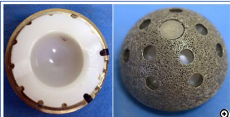
(Left) The acetabular component shows the plastic (polyethylene) liner inside the metal shell. (Right) The porous surface of this acetabular component allows for bone ingrowth. The holes around the cup are used if screws are needed to hold the cup in place.
